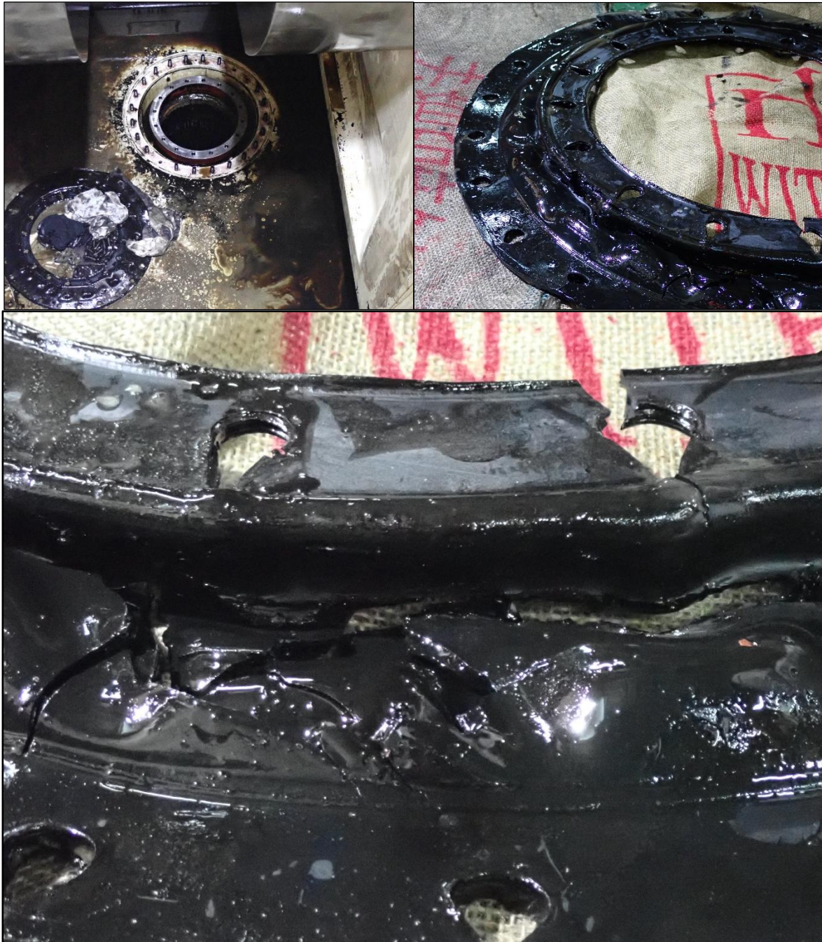
Figure 7: One of three rubber diaphragms removed from main engine sump.
